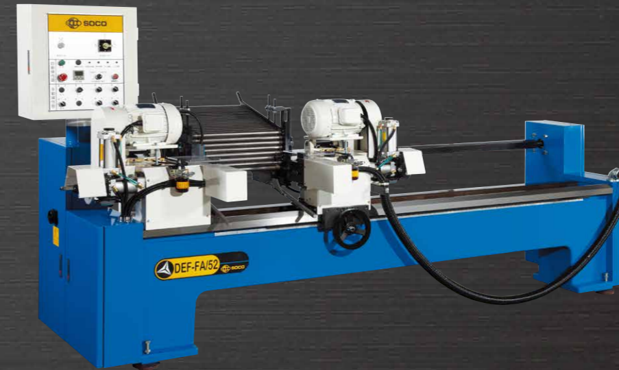
DEF-FA/52 Double Tubes Ends Chamfering for Working Lengths from 150 mm to 2000 mm. Capacity up to Ø52 mm. Fully Automatic Loading, Feeding and Chamfering.
